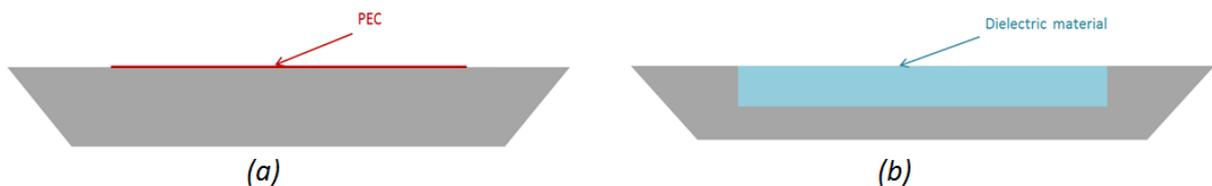
Figure 3: Reference case (a) and cavity filled with acrylic (b)
