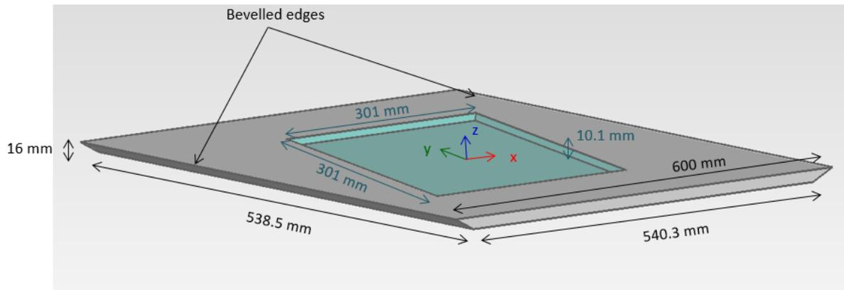
Figure 1: 3D structure and cavity dimensions
