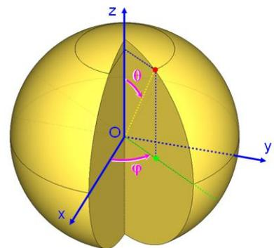
Figure 4: Definiton of the spherical angles
