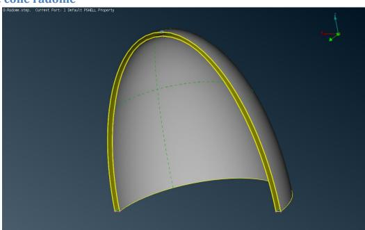
It is a 3-layer structure, with the following **nominal** material characteristics:
