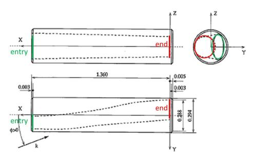
• The location of  $(y_{x}, z_{x})$  center of the section is a function of x :
