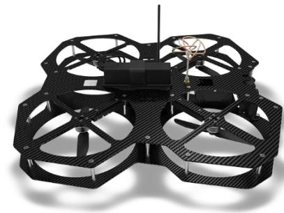
*Indoor drone with thermal camera*
