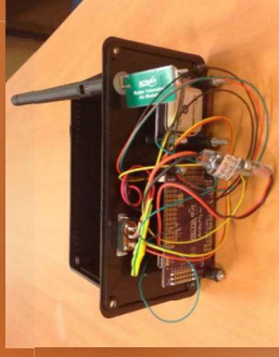
Flight controller of the AR Parrot UAV
