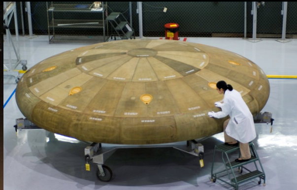
Orion heat shield ( \varnothing 5m)
