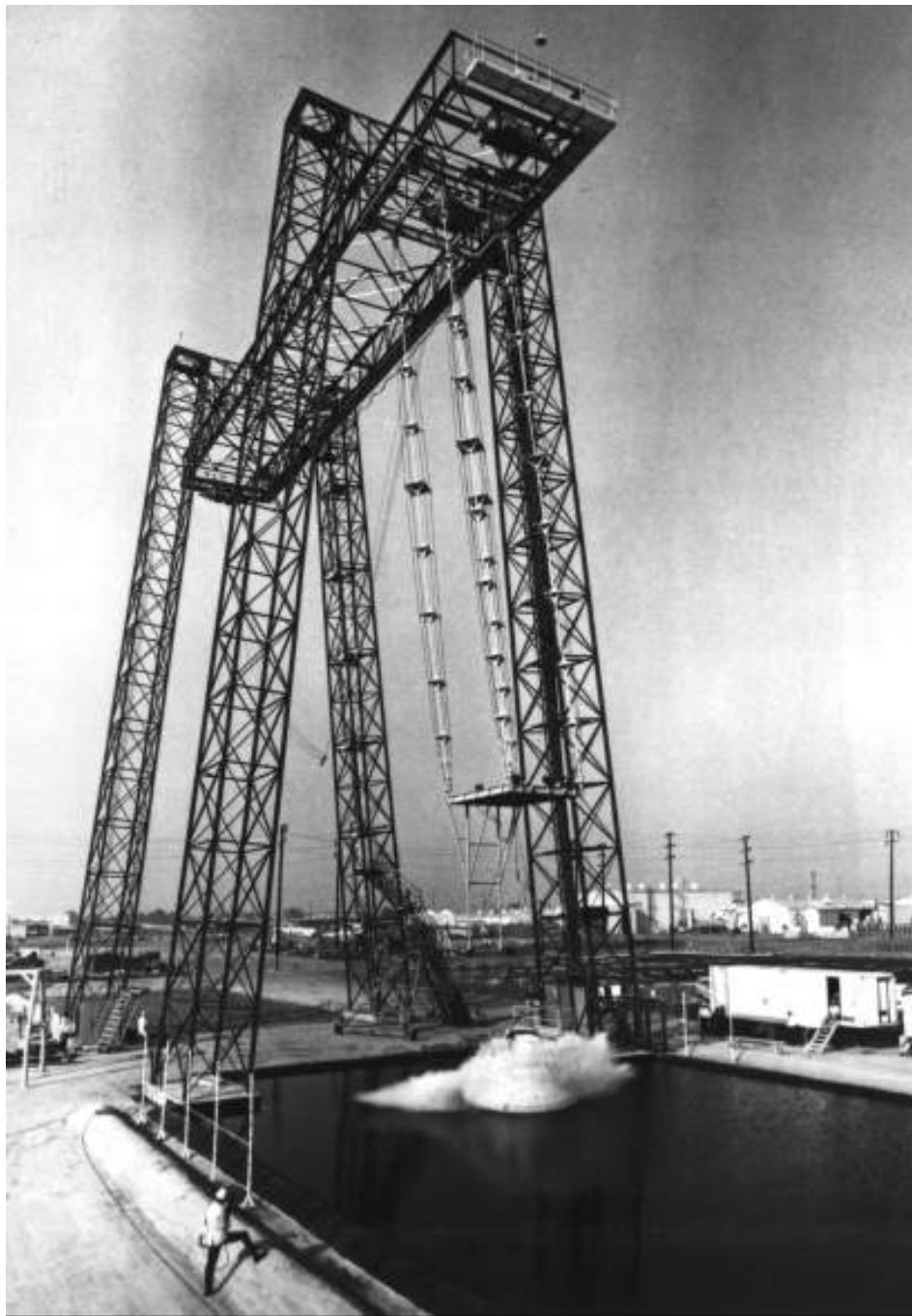
Full-scale splashdown tests at North American Aviation
