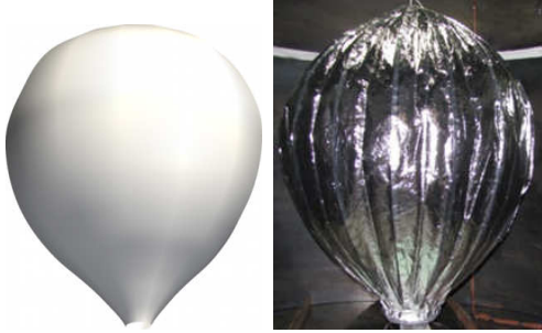
Fig. 5: Comparison of numerically rebuilt (left) and cryogenic tests real balloon.
