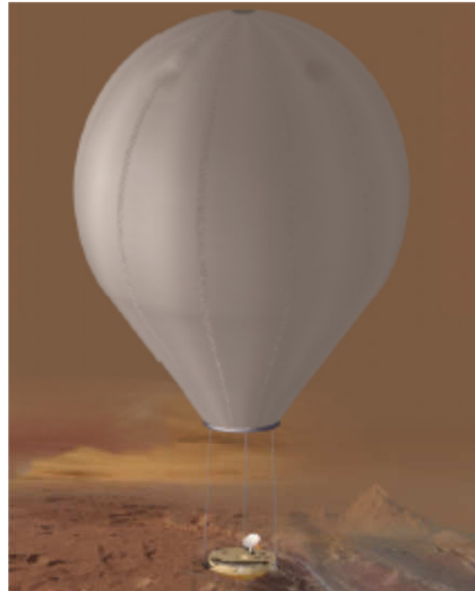
Fig. 1: Artist's concept of a double-wall Titan Montgolfiere balloon for the TSSM mission. [5]
