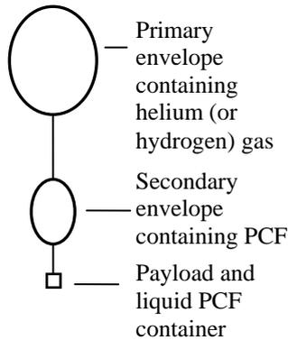
Fig. 2. Schematic of Tandem PCB
