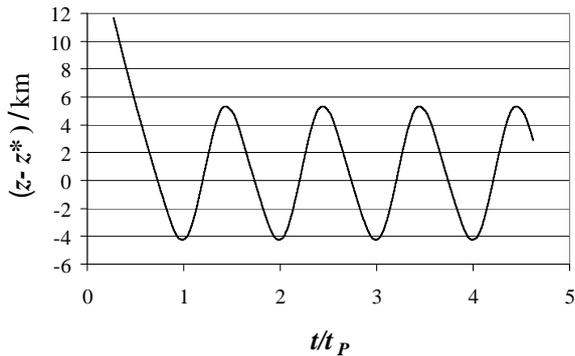
Fig. 3. Simulated Oscillations of Tandem PCB,  $z^* \cong 42 \text{ km}$ ,  $t_p \cong 11900 \text{ s}$  [3]
