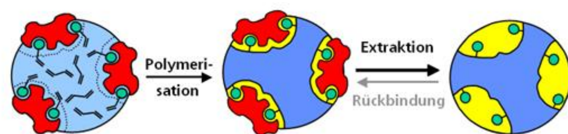
Figure 2. The MIP working principle (courtesy University of Stuttgart)
