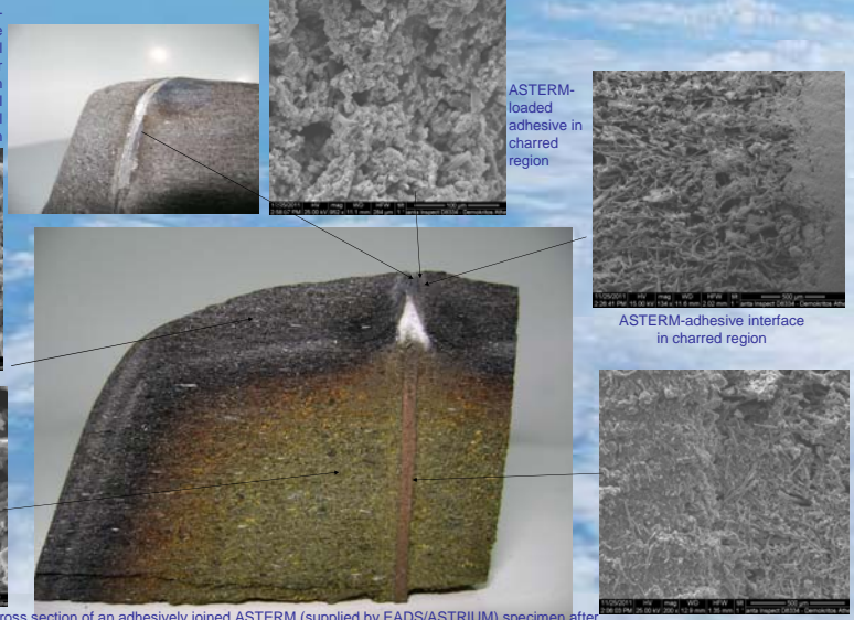
Cross section of an adhesively joined ASTERM (supplied by EADS/ASTRIUM) specimen after Plasma jet testing at 5MW/m 2 for 12 seconds at the Sirocco facility at CIRA. Total recession at top is about 2mm, it is fairly uniform and <0.5mm on the sides. Charred region varies from 6 to 12mm. Recession of the adhesive is slightly larger (photo on top left). The adhesive used was an RTV Silicone elastomeric rubber mixed with small amount of ASTERM powder
