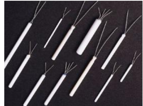
Example PRT: ceramic wire wound
