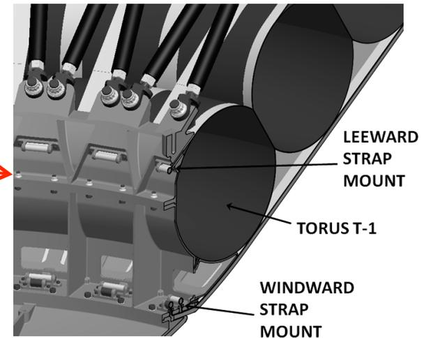
**Attachment of Inflatable Structure to Rigid Structure**
