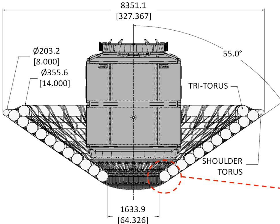
Torus – Braided Kevlar™ for structure; Silicone bladder for gas retention; RTV film for adhesion and sealing
