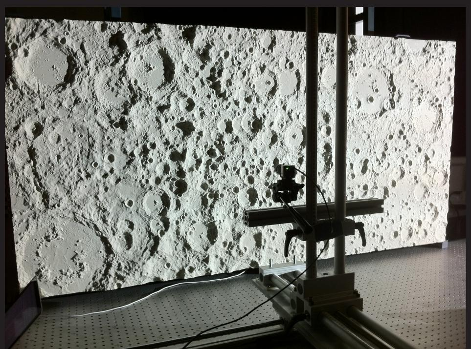
A 2  $m^2$  planetary mock-up based on NASA LRO lunar altimetry data was designed and set up at ESA-ESTEC. A 1024x1024 USB camera mounted on a static support and equipped with a lens providing a 75-deg field of view was used for hardware-in-the-loop tests. Ground truth accuracy is 2.4 mm and 0.2 deg (3 $\sigma$ ).
