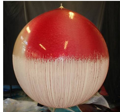
Fig. 6. Drizzle experiment using 0.7 m latex balloon using red-dyed water, showing transition from sheet flow to trickle flow, courtesy of Nevzat Atakan, see acknowledgements.
