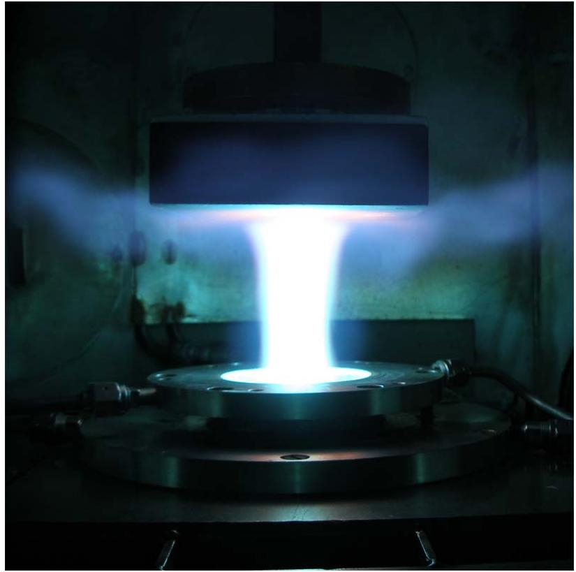
Thermal protection tile in carbon dioxide flow
