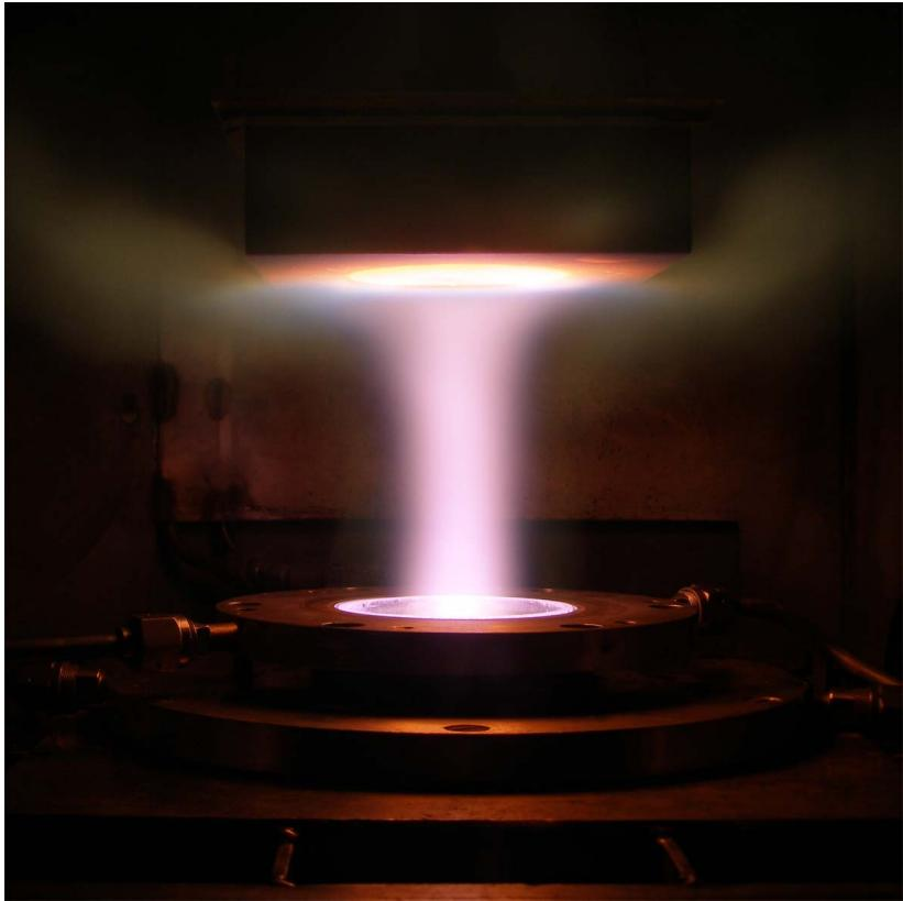
Thermal protection tile surface with catalytic ring in air plasma flow
