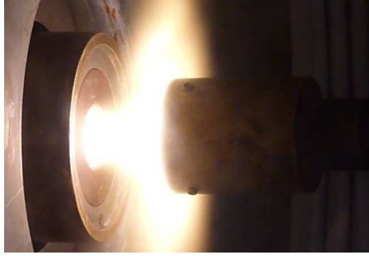
Fig. 1: Heat flux probe inserted into the pure nitrogen jet (a) and into the mixed nitrogen-methane jet (b)
