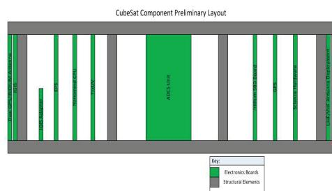
Figure 11: satellite basic schematics
