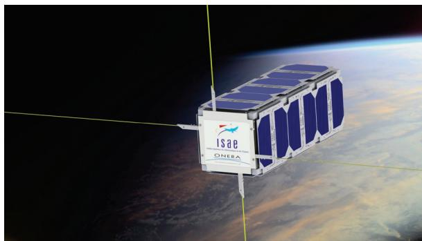
Figure 10: EntrySat CAD model
