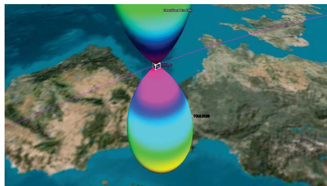
Figure 8: EntrySat Iridium antenna radiative patterns
