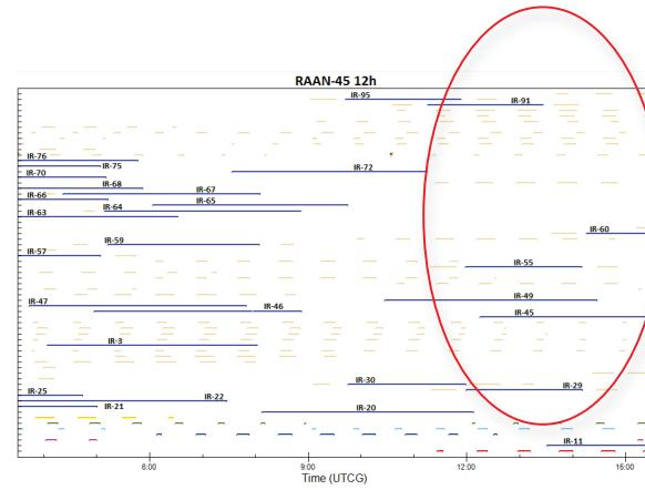
Figure 9: EntrySat – Iridium Access is possible with several satellites during the last 15 hours of predicted orbit
