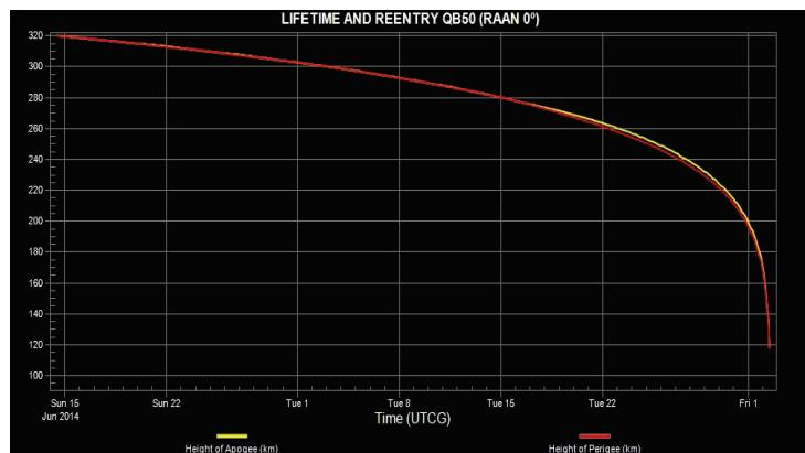
Figure 6: Projected satellite altitude for orbit of RAAN 0° Inclination 79
