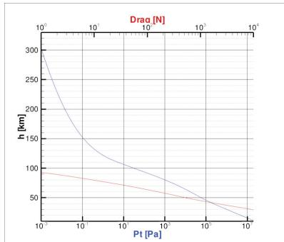
Figure 4 Drag force and maximum pressure during atmospheric re-entry
