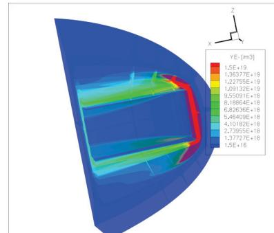
Figure 5 Electronic density around EntrySat during re-entry
