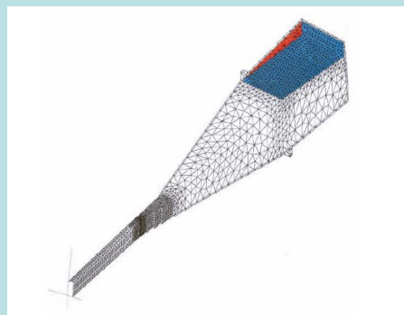
Pyramidal Horn With Dielectric Slab And Transition ORANGE LABS (F)
